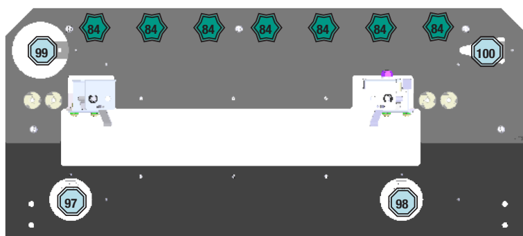
Figure 3.2.5. Playfield back panel lighting locations.
